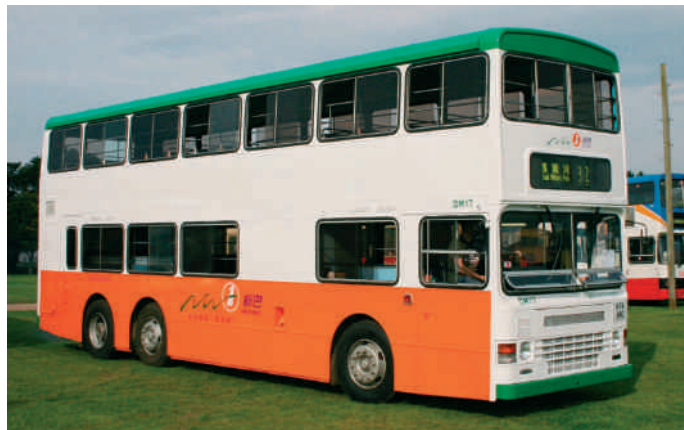
The former New World First Bus Dennis Condor with Duple Metsec body had seating for no less than 110 passengers.
