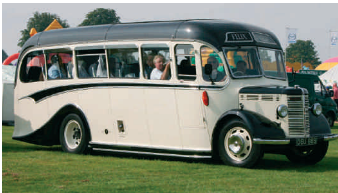
Felix of Long Melford entered this 1947 Bedford OB. The Duple body has 27 seats.
